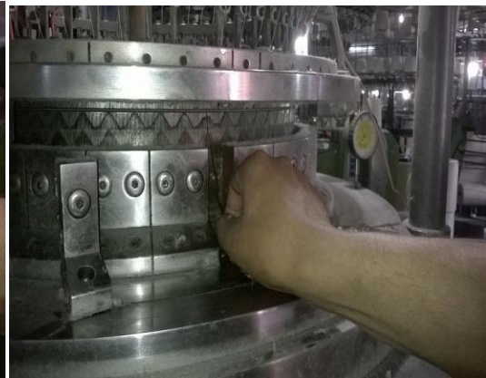
8 new needle inserted
