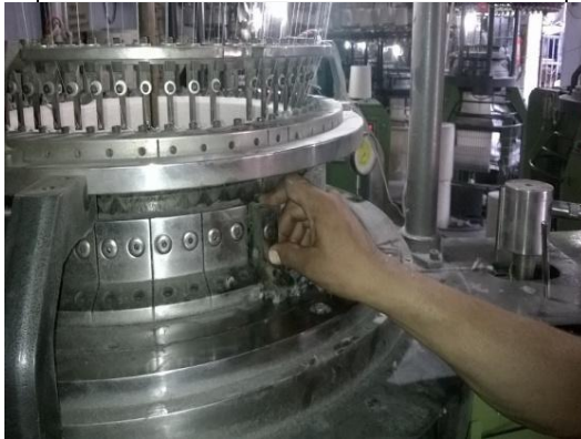
9 Needle holder assembled back
