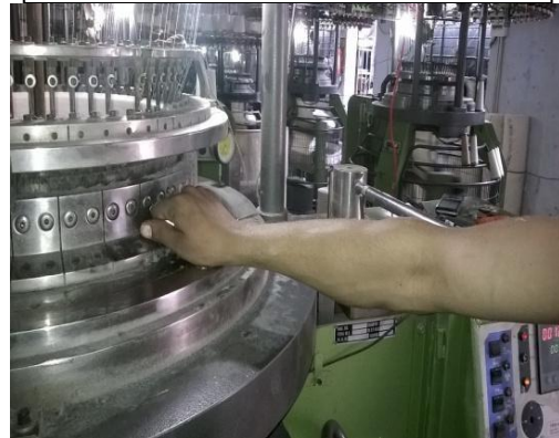
10 Needle holder assembled back
