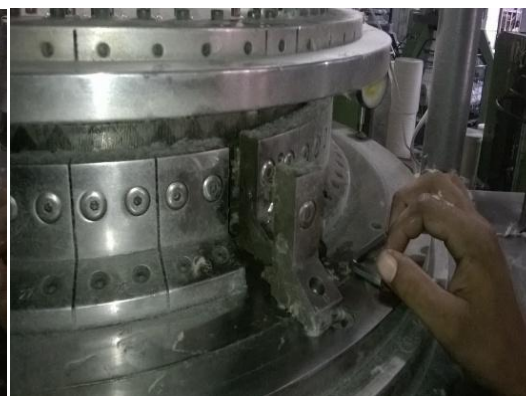
4 Needle holder pulled out
