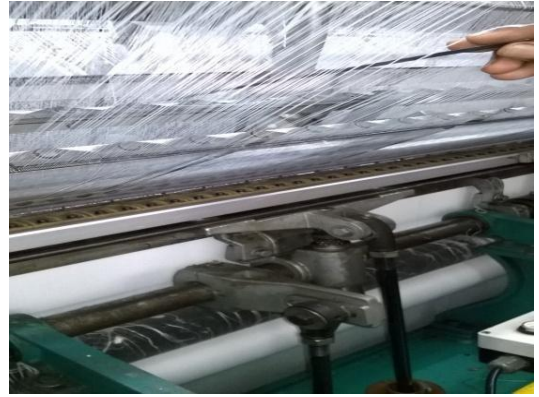
4 Thread passed through guides
