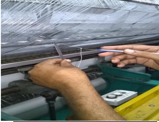
3 Broken thread gripped by hook
