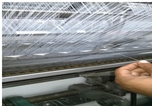
2 Broken thread is identified
