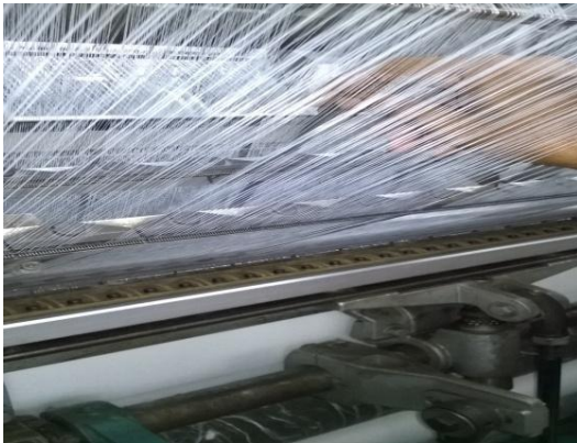
7 Thread passed through guides
