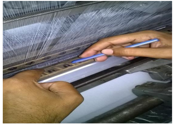
6 Thread passed through guides
