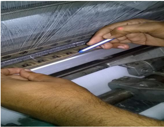
5 Thread passed through guides
